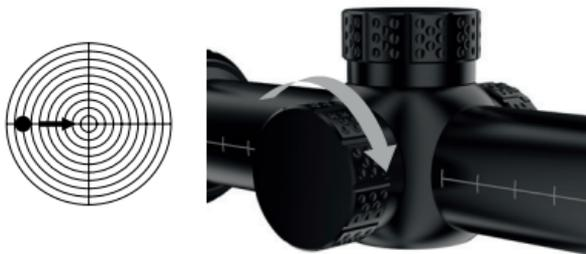
3. Unscrew the cap of the windage (side) turret. If the center of the group is 10 cm to the left of the center line of the target, then the group needs to be adjusted right (windage) 10 cm. 1 click will move the group 1cm 100 meter, so 10 clicks will move the group 10cm at 100 meter. Adjust the turret in the specified direction you want the bullet group to move.
